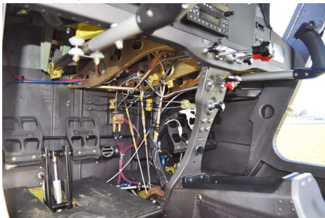
"The dark grey paint scheme and lack of trim give the interior a rather industrial appearance" with no attempt to hide the workings. The control sticks are a real departure from normal Cessna practice.
